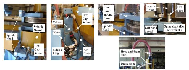
8.9.9. Remove the handle from the head and tie it from the arm of the front control panel so as to not put tension on the air line to the handle.
